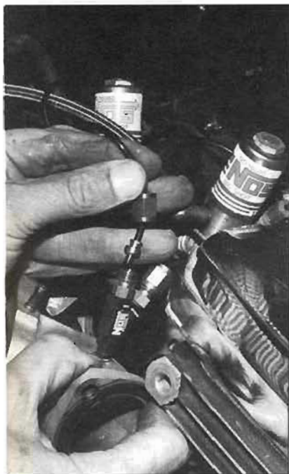
Here, the nylon fuel line, which feeds the fogger nozzle, will be threaded onto the solenoid with brass compression fittings.
