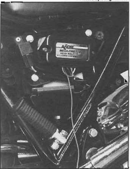
The adjustable Accel ignition, Mega Fire module installed in the same location as the stock unit.
