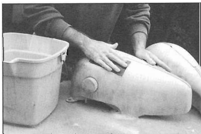
Primer builds thickness and block-sands (with 500-grit wet and dry) easily. Palmolive dish soap prevents fingerprints and clogging.
