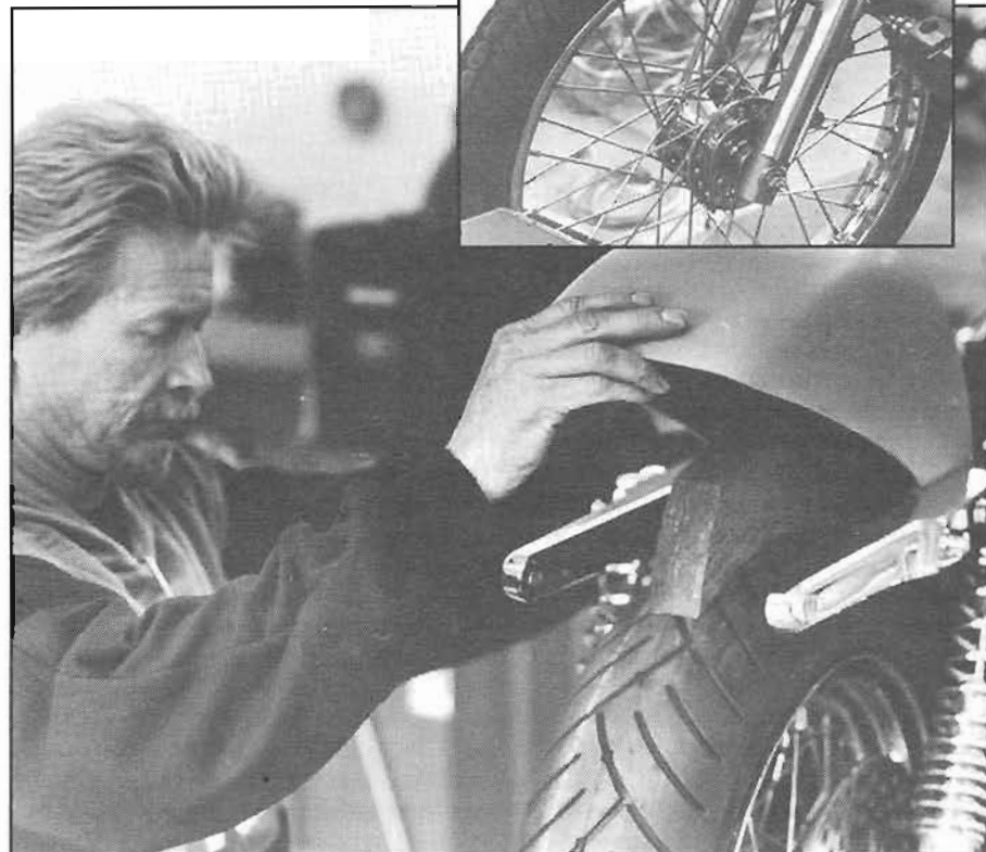
Arlen positioning fender on wood guide.
