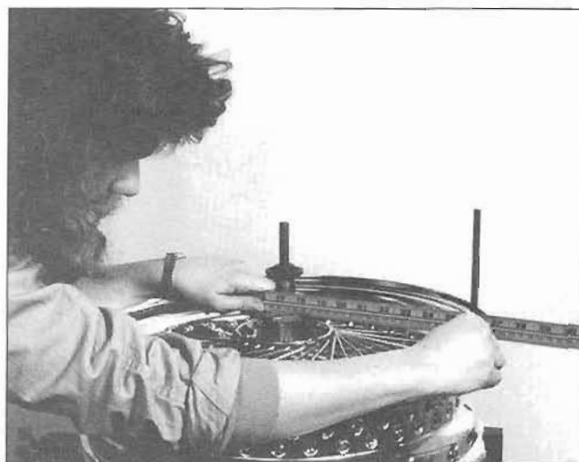
With all 80 spokes loose in the rim, Brook uses a straightedge to set the required offset of the hub to the rim.
