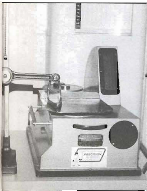
This demonstrates how the reciprocating end of the rod is weighed.
