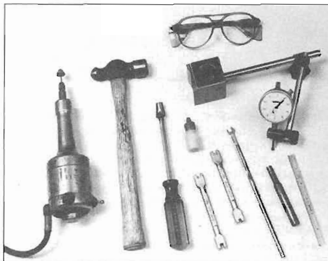
Hand tools needed to complete a wheel. Brook had to make her spoke wrench to work on an 80-spoke wheel.
