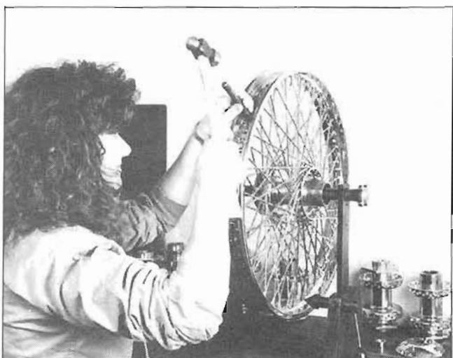
After the wheel is trued, she sets the nipples into the rim. The wheel will probably have to be retrued after this step, but it will stay true during use.
