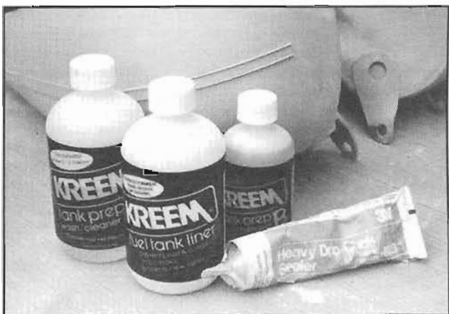
Tanks were coated with Kream to prevent rusting and leaks. Because of acid, this should be done before primer.
