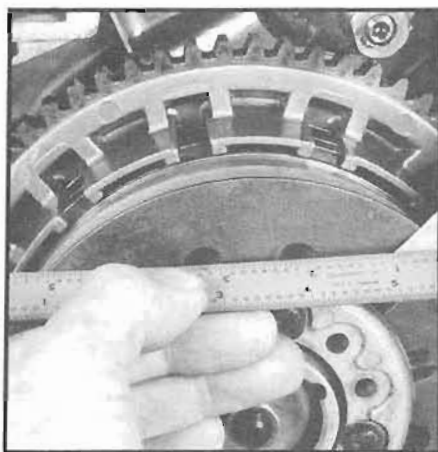
Clutch spring shape can be measured with ordinary tools. Note that the four spring retaining bolts are fitted through holes with a letter—either A, B, or C. These hole sets pre-load the spring different amounts, changing its shape. Best lever feel results when the spring is flat or slightly dished (left photo). The large contact area of the new clutch hub eliminates wear and the sticking between the plates and hub.
