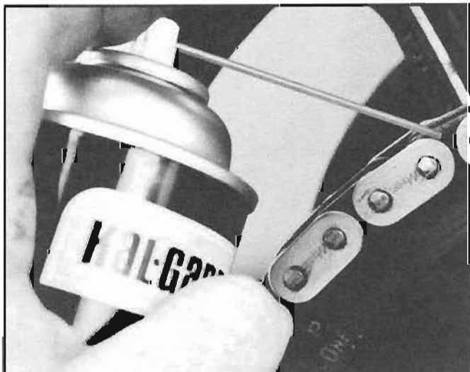
Squirlin' lube all over the outside of yer chain won't help much — it's gotta get inside. All them Harley power-pulses go through the pins and bushings inside the chain.
