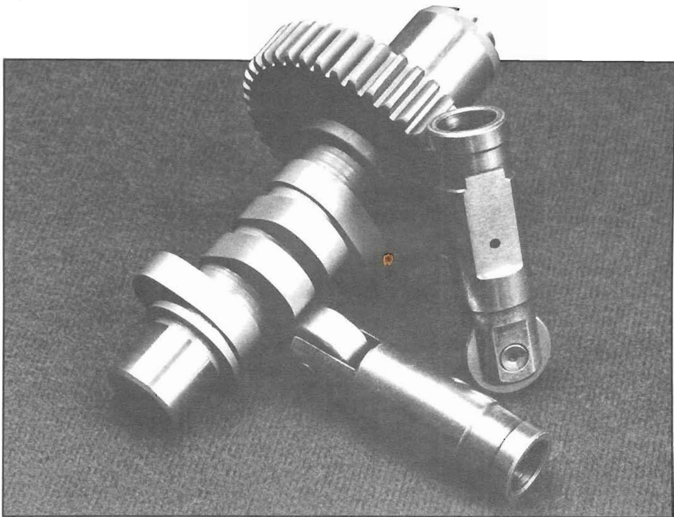
For good, lasting performance the Andrews "J" or "A" grind cams work well with standard hydraulic tappets.
