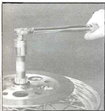
Axle nut must be torqued correctly when measuring end play.
